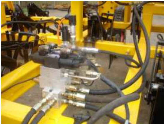
▲ Hydraulic manifold mounted to the Multiplanter.
