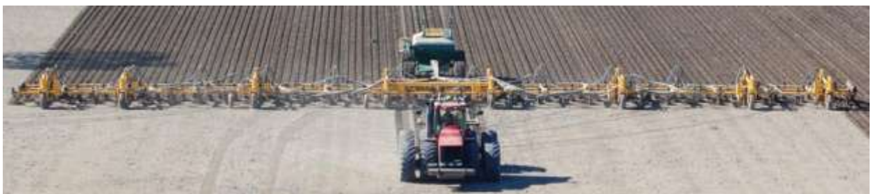
▲ The Case STX500 500hp pulling this 160ft (48m) Multiplanter went from 100% to 65% tractor power with the sensor tine fitted. This is over and above the savings achieved by depth controlling the digging tip. Photo courtesy of Wallaby Productions.
