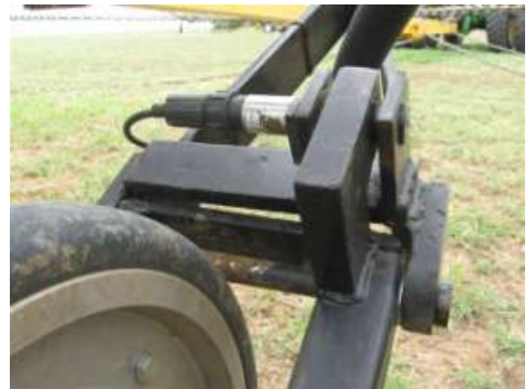
▲ Load sensor pin fitted to the master hinged press wheel fork.
