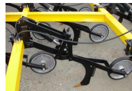
◀ Parallelogram controlled tyne assembly with 2" spear tip.
