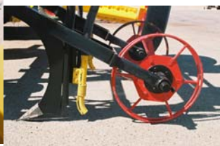
▼ Tyne assembly with spring steel press wheel.
