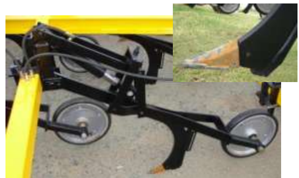
▲ Multiplanter tine assembly with 2" (50mm) spear tip.
