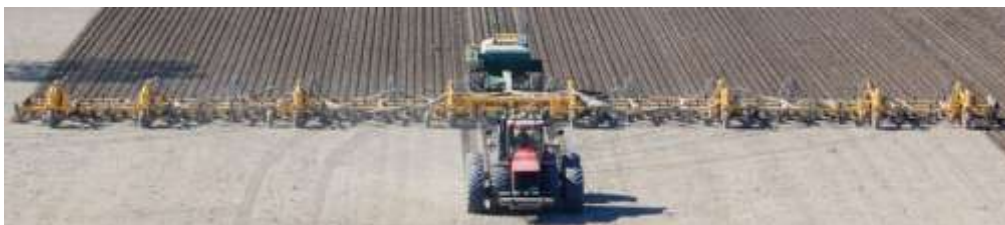
◀ 160ft (48m) Multiplanter has sown down to depths of 9" (228mm).
